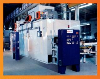
**WOOD PRODUCTS -** Gas-fired, high velocity convection oven for curing water borne coatings on exterior wood siding. Cure time: 6 seconds at speeds of 400 fpm.
