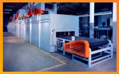
**FOUNDRY -** Multi-zone conveyorized convection oven and cooler for curing water-based coating on sand cores.
