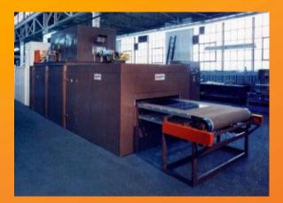
**SILK SCREEN -** Electric radiant and electric convection oven with cooler to process metal, vinyl and fabric silk screened substrates.
