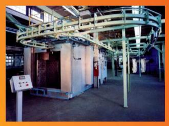
**SPECIALIZED CONVEYOR OVENS -** Gas or electric ovens with special conveyors including loaders/unloaders and cooler for electronic parts, air bag housings, plastic parts and special castings.
