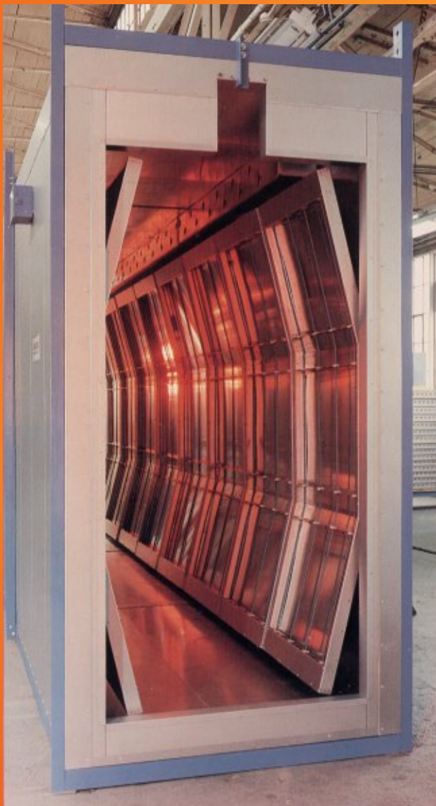
Conveyorized electric infrared oven; interior shaped to suit part.
