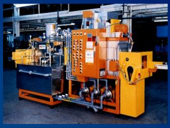
**AUTOMATIC IN-LINE PROCESSING -** Tooling fixtures are diverted to this 2-Stage combination washer/drier then returned to the production line.
