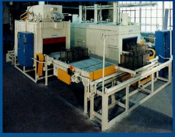
**AUTOMATIC BATCH PROCESSING -** Baskets of parts are cleaned in a 3-stage process and dried in an integral oven.
